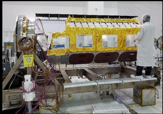
L-SAR MLI being installed for upcoming TVac test
