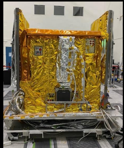
KaRIn Module Ready for TVac Test in 10' Chamber
