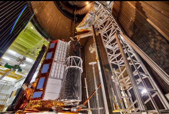
NISAR Dynamic Test Model (DTM) in 25' Chamber
